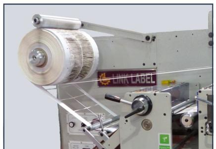
Link Label's rewinders are designed to work in line with their printing machines, hot stamping machines or die cutting machines.
